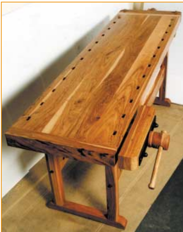
🔧 A teak 2m-long versatile cabinet-making workbench.
